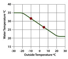
outdoors, the heat output of the boiler will be decreased. For example when it is -10°C outside the water temperature will be 32°C, and when it is 5°C outside the water temperature will be 27°C.
